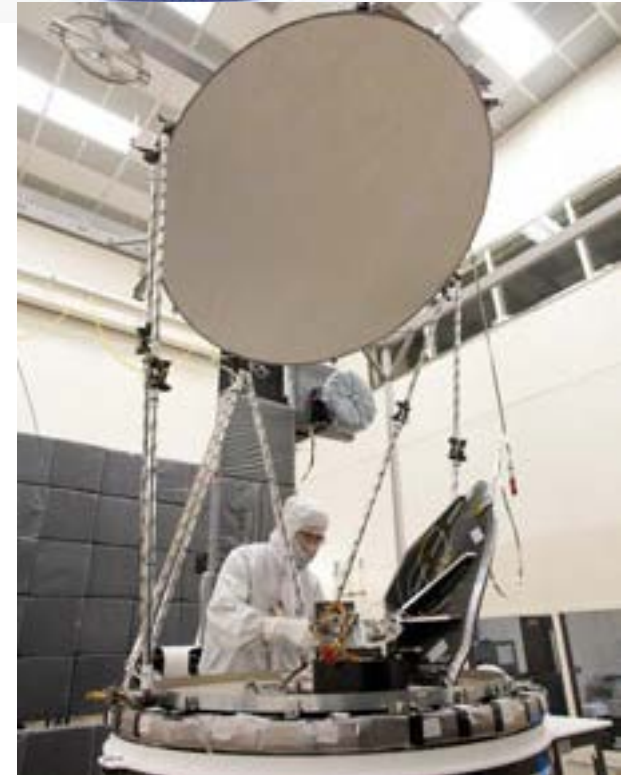
A test technician completes the final electrical integration of the GMI. Credits: Ball Aerospace
