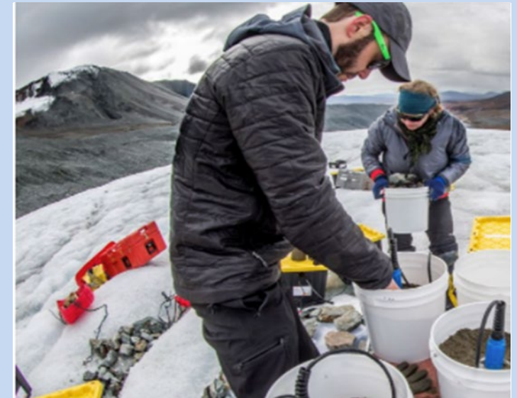
Brad Averson, an engineer with Silicon Audio, sets up seismic sensors on Gulkana Glacier in Alaska to see if a NASA lander would work on icy Europa.
