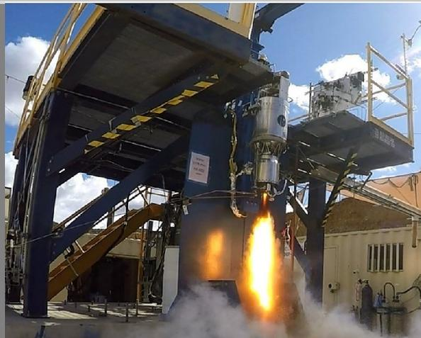
**Parabilis Space Technologies** developed a hybrid stage that combines the benefits of traditional liquid and solid propulsion systems while reducing risk and cost. Parabilis received additional funding from NASA and the U.S. Air Force to develop this technology beyond the Phase I and II STTR accomplishments. <https://go.nasa.gov/2XeYbDA> [17]
